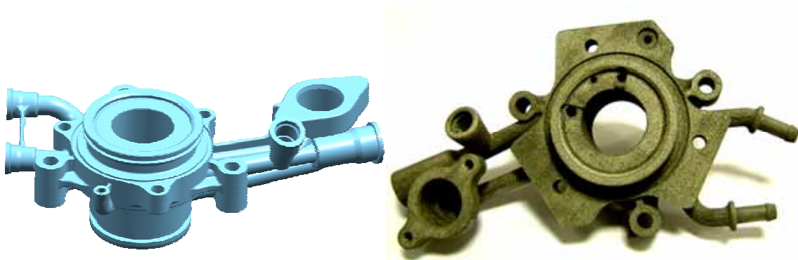
Figure 6. Re-designed front-plate component (left) and an example manufactured using SLM (right)
