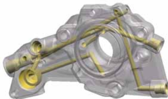
Figure 2. Original diesel front plate design, grey areas show main body casting, yellow areas are machined diesel pathways
